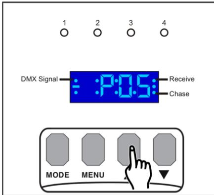
2. Set you desired chase pattern: Once you have selected the chase function use the Menu button to select your desired chase. The chase pattern is represented in the LCD display by "P" followed by two numbers. You may select any of the built in 16 programs to run at a single time.
