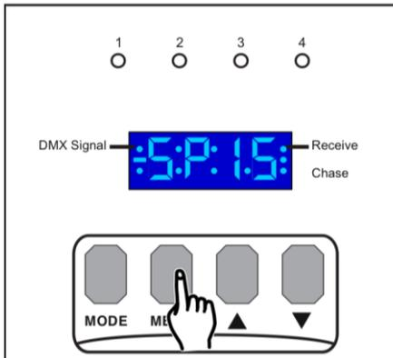
3. While in chase mode, tap on the MENU button until the "SP" followed by two numbers is displayed in the LCD. Press MENU to enter Chase Speed mode.
