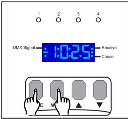
4. Press MENU to set the DMX address for the desired channel. Tap ▲ or ▼ to select the desired DMX address 001-512.
